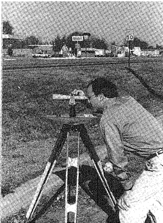
Louis J. Driber, USGS, uses a plane table and alidade in level line surveying.
