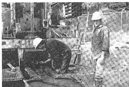
Scott Andres and Tracy Stapleford collecting samples of drill cuttings from the mud pit.
