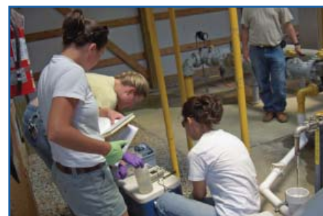
Staff members (from left) Hilary Gittings Trethewey, Liz Wolff, and Muserref Turkmen measuring pH and specific conductance of treated waste-water effluent at the Landis Sewage Authority, near Vineland, New Jersey.
