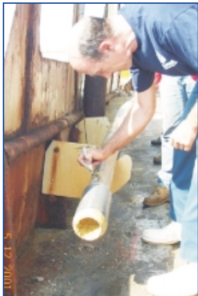
Crew member from Alpine Ocean Seismic Drilling Norwood, N.J. labeling a core on deck of RV Atlantic Twin. Funding for collection of the cores came from the Minerals Management Service.
