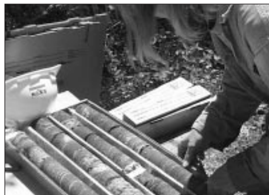
Cores of weathered crystalline rock (saprolite) from 454-463 ft.
