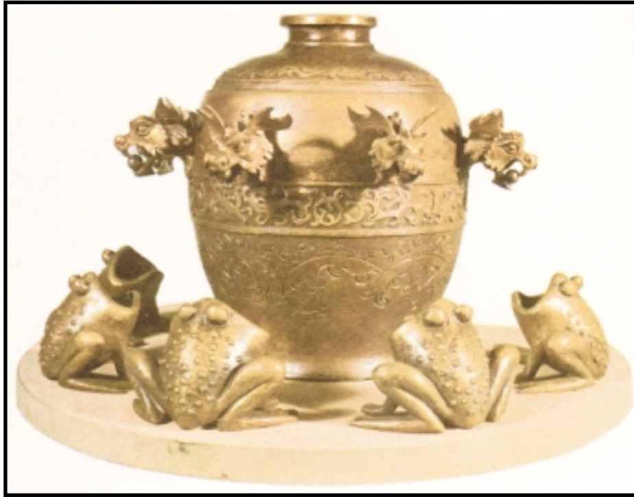
Figure 6. Model of earliest seismoscope invented in 132 A. D. From U.S. Geological Survey web site http://wwwneic.cr.usgs.gov/general/handouts .
